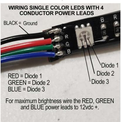
positive. The point is that with a four conductor power lead on a single color LED strip, you have some flexibility as to controlling brightness.
