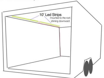
In this example, the power leads (red dashed line) from each LED strip follow the roof line forward to the corner and then down through the floor where they attach to the power source and/or LED controller.
