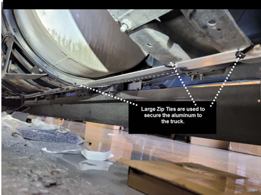
A close up view of how we mount the aluminum flat bar to the truck's sub-structure
