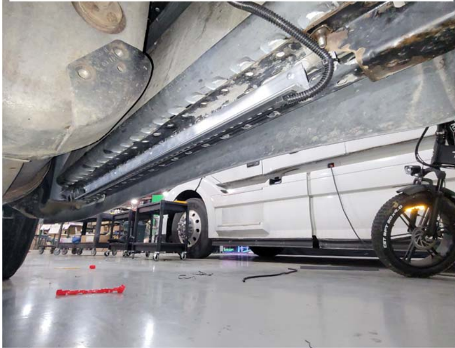
View of LED Segment 'E'. Mounts to the 33" plastic 'L' angle (aluminum angle not used as shown in this photo).
