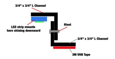
The Passenger's Side Z-Bar needs to be 30" long. The Driver's side doesn't use a Z-Bar. It uses a single L channel. This is a view of the passenger's side LED strip mounted to the Z Bar.
