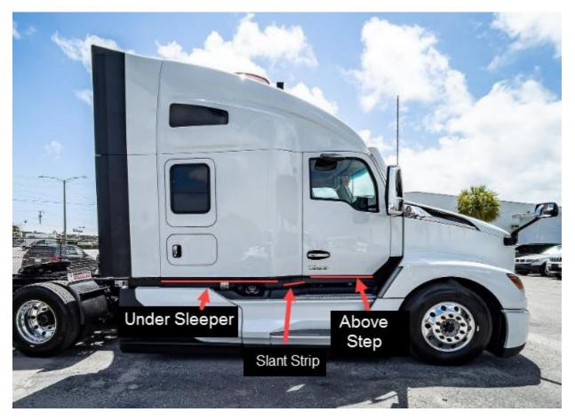
The LED strips that mount under the cab (above the steps) on both sides of the truck need to be mounted on the supplied  $\frac{3}{4}$ " x  $\frac{3}{4}$ " plastic L channel. The passenger's side requires a 30" 'Z-Bar' be crafted using two pieces of  $\frac{3}{4}$ " plastic that are riveted together (see below diagram). The driver's side uses a single 24" long  $\frac{3}{4}$ " x  $\frac{3}{4}$ " L channel.
