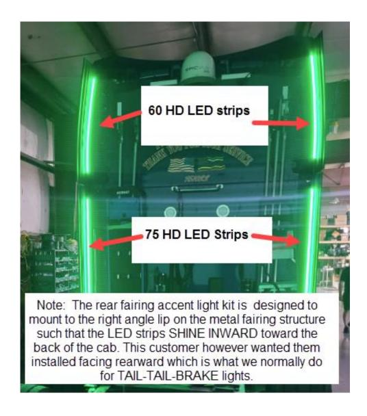
**Tail-Turn-Brake (TTB):** If you also purchased the Tail-Turn-Brake light kit these LEDs are mounted on the back of that right-angle lip facing toward the hitch/trailer/traffic behind you. In this situation, the RFA LED lights can only be mounted facing toward the back of the cab since the TTB lights are mounted on the other side of that metal lip.
