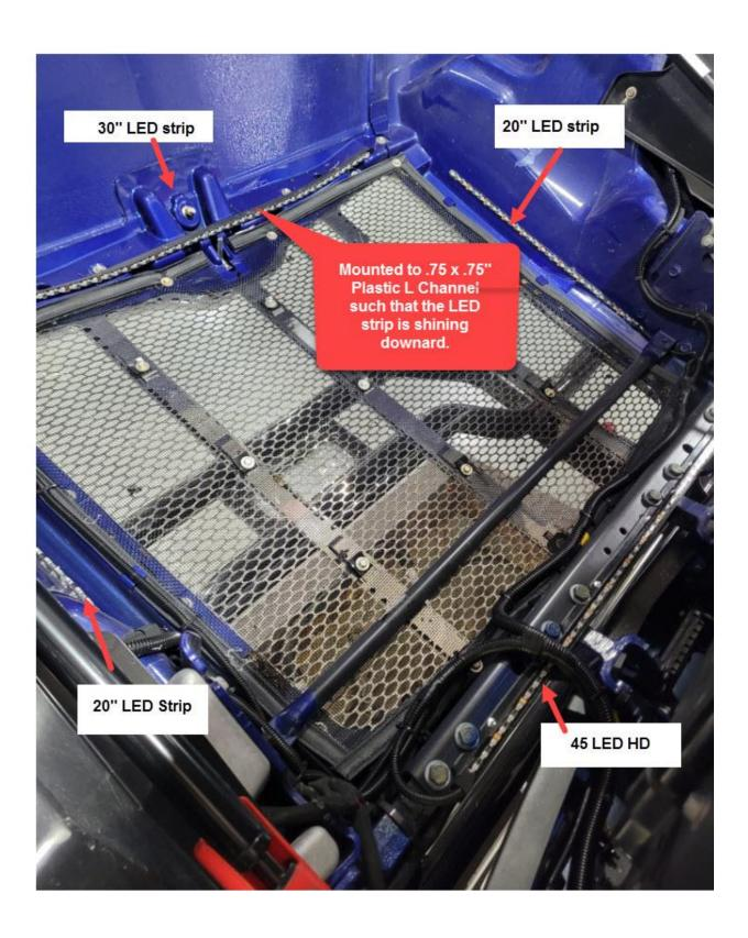
Note that if you're also installing our AIR VENT light kit, we suggest wiring the Air Vents together with the Grill Light. We say this assuming you want both light kits on the same lighting zone. If you
