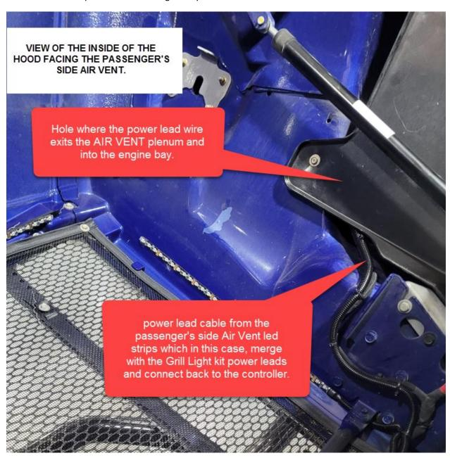
Note that if you're also installing our GRILL LIGHT kit, we suggest wiring the Air Vents together with the Grill Light. We say this assuming you want both light kits on the same lighting zone. If you purchased a dual zone LED controller then you have the option of wiring these two light kits on separate zones. Personal choice.
