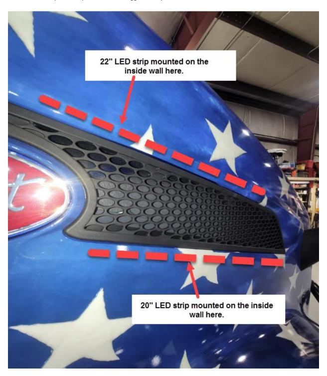
You'll need to drill a hole on the inside of the hood to pass the power lead wire though. Since it's a plenum, you'll want to make sure you seal that hole. We use Lexel but any silicone sealant will work. Be sure to wrap the power lead with split loom too to stop the power lead wires from chaffing. Note that we prefer to wire the two LED strips together inside the air vent plenum and then only have one power lead wire exit that plenum into the engine bay.
