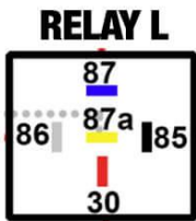
view of bottom of relay each pole is numbered
