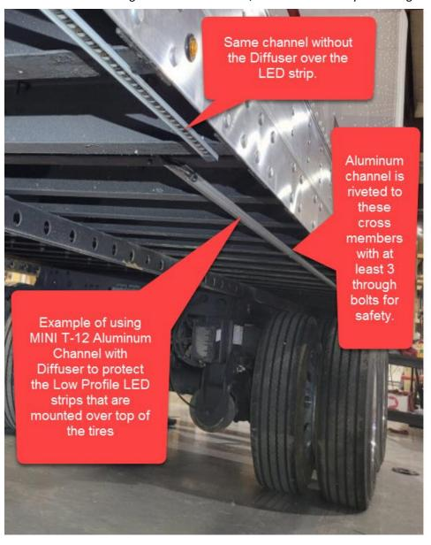
This photo is from a double axel travel trailer. We installed the aluminum flat bar to the bottom struts and then mounted the LED strips to that aluminum flat bar.
