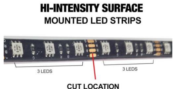
The LED strip can be cut one time on the copper solder pad where indicated; between the cluster of 3 LEDs. Important to cut in the center of the copper pads. Once cut, the end must be sealed using silicon, liquid electrical tape or even heat shrink to stop water intrusion from damaging the strip.
